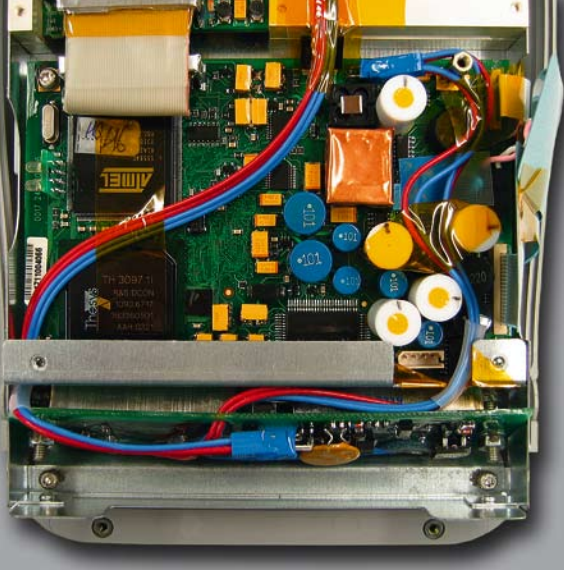
FIG 4 Ready for a trip to space: the R&S®FSH3 after modification. Especially materials containing PVC and electrolytic capacitors could endanger the astronauts and thus had to be replaced.
