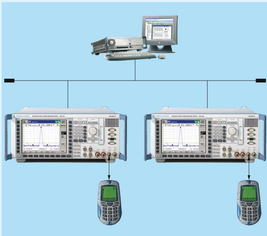
FIG 5 Test setup for data end-to-end tests, for example for testing the exchange of an MMS message between two mobile phones.
